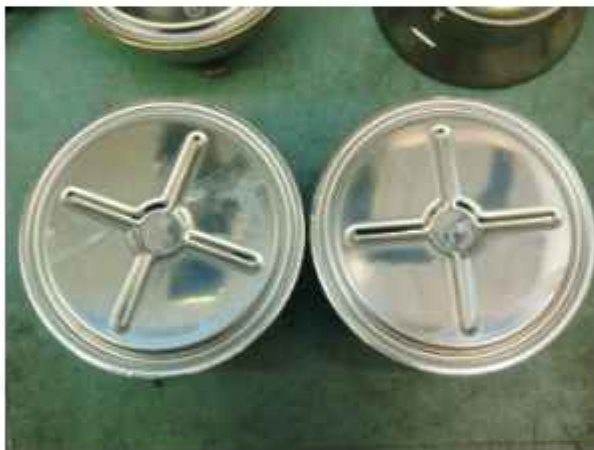
Function: circular welding of AISI 316L steel component Component type: Coffee maker base
