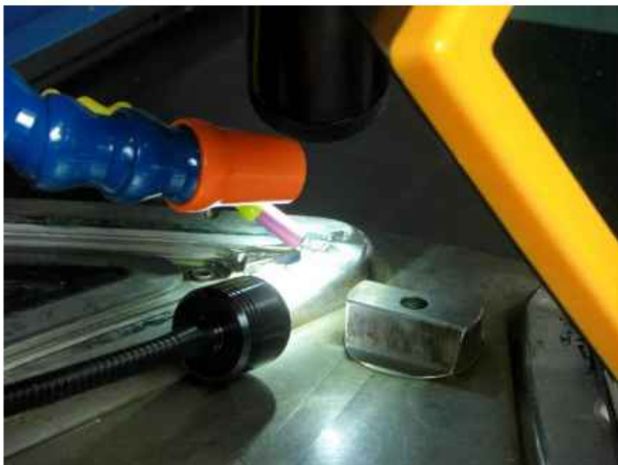
Repair of mould for rubber injection
