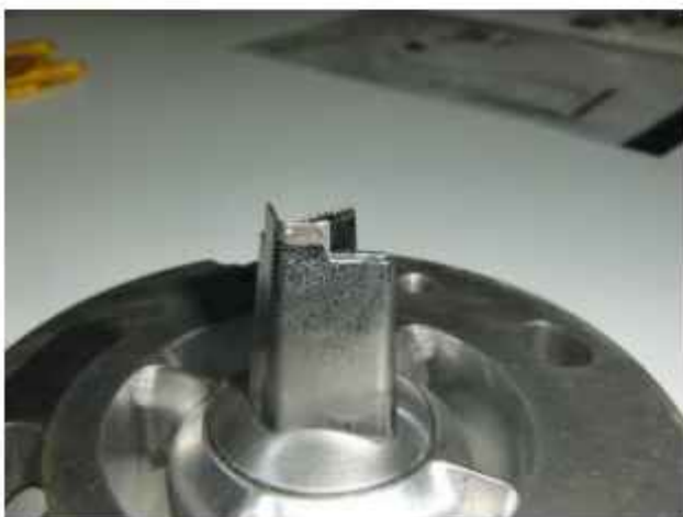
Process: Reconstruction of wall with thickness 0.3 Mould type: Plastic moulding
