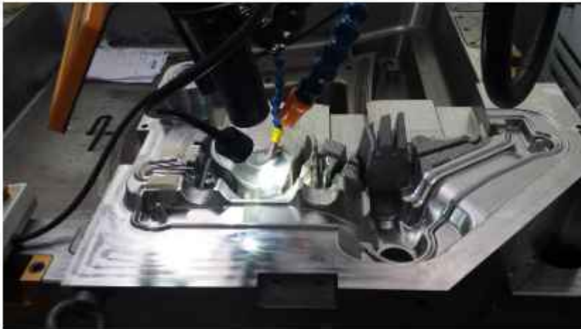
Process: Reconstruction of a damaged area Mould type: Die casting
