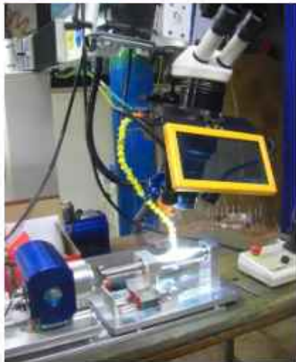
Function: Circular welding on steel Component type: Pressure switches
