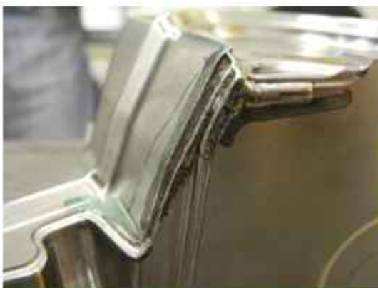
Process: Reconstruction of a damaged area Mould type: Die casting
