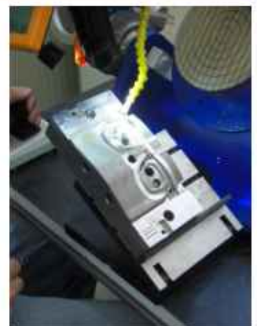
Process: Repair of an inclined surface Mould type: Plastic material mould
