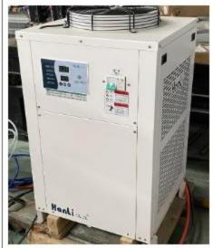
Brand:wuhan hanli chiller Cooling the laser and cuttinghead Dual temperature and dual control
